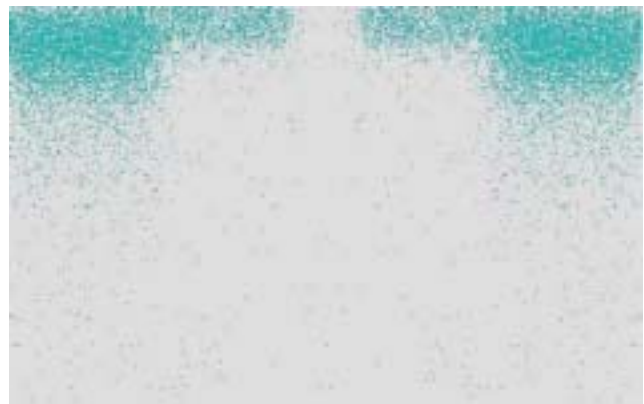
Figure 4: Source and drain profiles after 15 seconds anneal at 950^\circ\text{C} .
