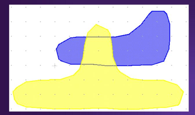
Images on photoresist (i.e. "silicon layout") are saved as mask files in Prospector and then transferred to Taurus-Process for the etch modeling
