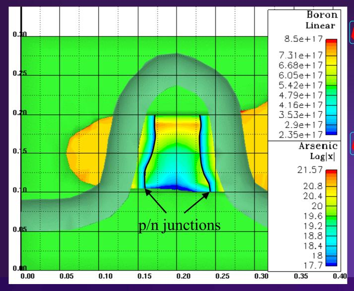
Electrical channel length varies from 60 to 85nm across the channel
