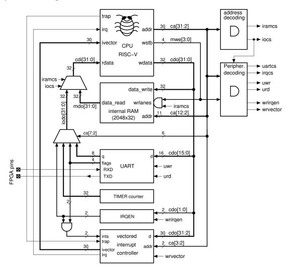
The above figure shows the block diagram of the system, that basically includes a laRVa CPU, 8KB of internal RAM with a known initial content, and an small number of peripherals:
