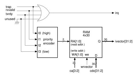
The diagram of the simple Vectored Interrupt Controller is shown in the above figure. The system has 3 possible interrupt sources, each of them with an specific interrupt vector (write-only) where the memory address of the corresponding interrupt service routine is stored. There is also an interrupt enable register that allows the selective masking of interrupts:
