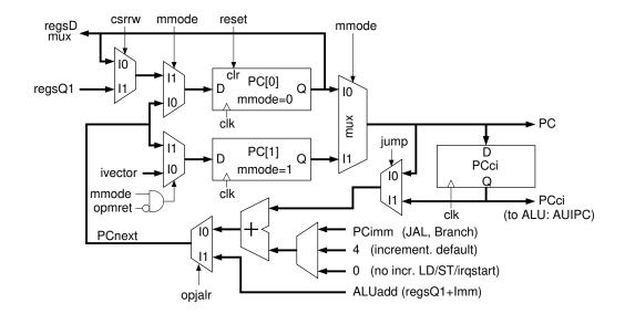
The "mmode" signal selects which register to present at the output, and also the values written back to each register. In normal mode (mmode=0) the register PC[0] is selected as output and it is updated every clock cycle, while the register PC[1] is written with the value "ivector", that is the address of the next interrupt service routine. In interrupt (AKA machine) mode PC[0] remains with it last value stored and PC[1] is presented at the output and updated.
