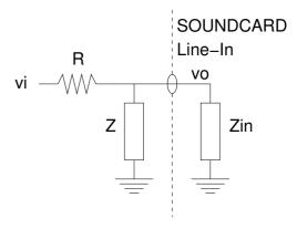
Figure 6: Setup for impedance Measurements.
