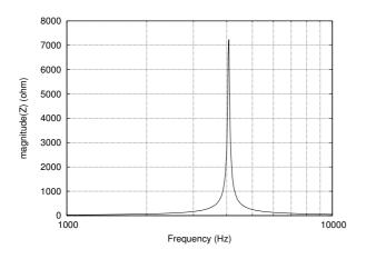
Figure 7: Measured impedance of the LC tank of the example circuit.
