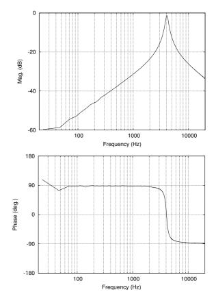
Figure 4: Measured Bode plot after delay adjust. No channel calibration.
