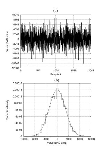
Figure 1: (a) Test signal. (b) Amplitude histogram and Gaussian fit (rms value: 2894).
