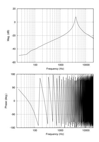
Figure 3: Measured Bode plot before delay adjust and channel calibration.
