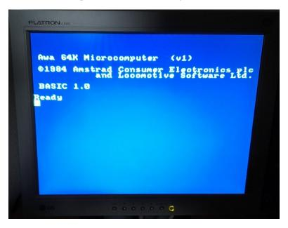
Well, the system at that point included only the video controller, the CPU, the memory, and the boot ROM and I/O. The rest of the peripherals were still missing. Interestingly, the manufacturer is listed as Awa, not Amstrad. Also the text color was cyan, not yellow as it should be. There was an error in the bit order of the pixels in video mode #1 that was easily detected and corrected.
