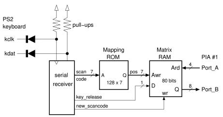
Unfortunately, the symbol to key mapping on the PET is quite different than that of the spanish PS2 keyboard, and some symbols had to be placed on unrelated keys (the hardware is fine, but some keys ought to be relabeled). Otherwise the keyboard works quite well.
