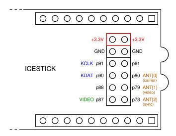
The signals discussed before are attached to the ICESTICK board pins at the positions shown in the above figure (upper side). A photograph with the board connected to a monitor and a keyboard is included next:
