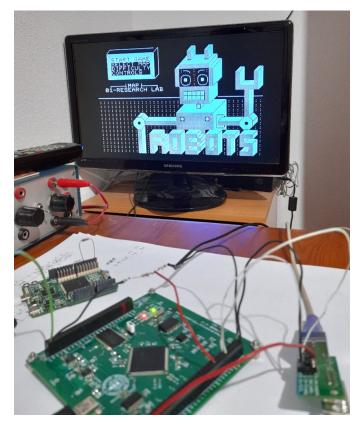
The support for uploading snapshots was also included in the "reduced" ICESTICK version of the PET, resulting in all BRAM blocks being occupied and only 5 unused logic cells out of 1280. That's a tight fit! The same small ICE40HX1K FPGA was also used in an old ICECREAM board but in that board we also get the external RAM. This results in a "reduced" 32K PET that is able to play PETSCII Robots without sound.
