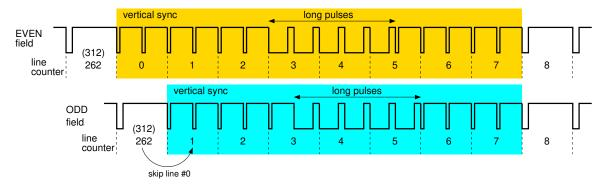
In our recreation the even and odd fields of the image show the same lines. This results in half the vertical resolution, but we only need 200 lines and a full resolution will result in the text being "compressed" vertically at the top of the screen. The displayed lines are placed at the middle of the screen and some top and bottom borders are left around the image.
