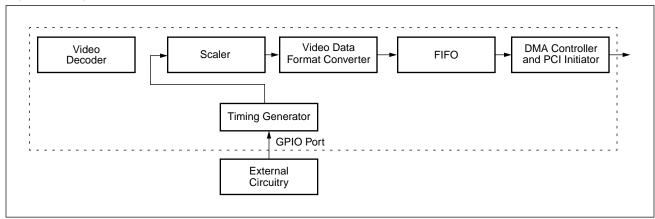
Figure 39. Asynchronous Data Parallel Port Interface
