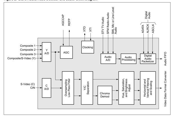
Figure 2. Bt879 Audio/Video Decoder and Scaler Block Diagram
