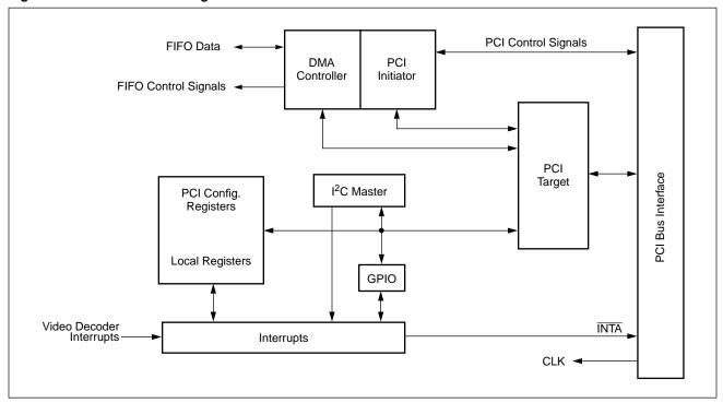
Figure 34. PCI Audio Block Diagram
