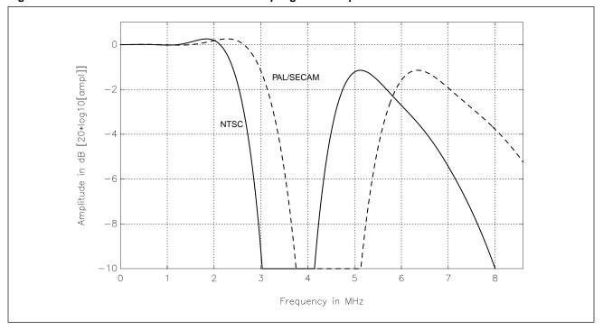
Figure 12. Frequency Responses for the Four Optional Vertical Luma Low-Pass Filters
