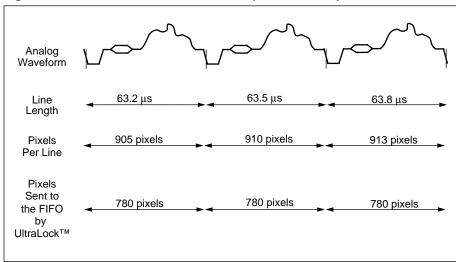
Figure 4. UltraLock™ Behavior for NTSC Square Pixel Output
