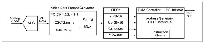
In the VBI frame output mode, the VBI data capture occurs in the active video region and includes all the horizontal blank/sync information in the data stream. This feature can be used to provide a high quality still-capture of video. The data is vertically bound beginning at the first line during VACTIVE and ending after a fixed number of packets. The data stream is packetized into a series of 256-DWORD blocks.
