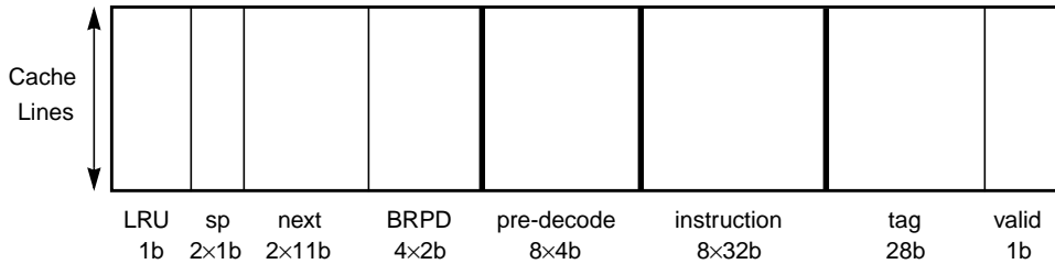
FIGURE A-4 Simplified I-cache Organization (Only 1 Set Shown)
