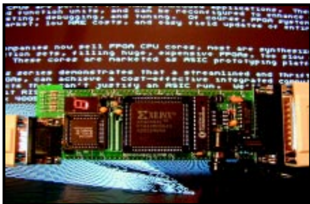
Photo 1—Here's the XS40 board, with the project design loaded into the FPGA and running a demo program that's drawing graphics on the monitor.
