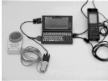
(PDA with DSP-100 installed, connected to a GPS system and a Geiger counter)
