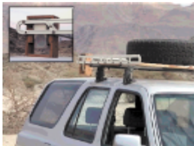
(Radiation mapping system mounted on a jeep)
